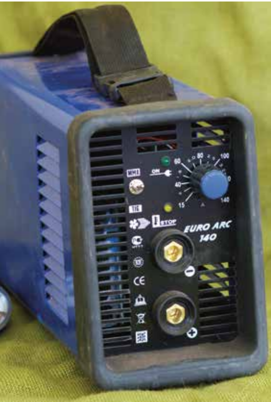
There are several basic inverter TIG welders on the market which can be purchased for a few hundred dollars. These machines are little more than a stick welder attached to some TIG components, and are DC only, meaning welding aluminium is not possible. They are severely limited, with no pulse function, and must be 'scratch started' to initiate the arc.
