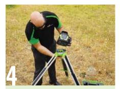
Attach the level to the tripod using the bolt through the base plate. Make sure the unit is reasonably level.
