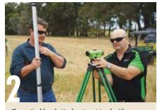
The optical level attaches to a tripod with a domed top. Make sure the tripod is located on stable ground and the spikes on the legs are well pressed in. Adjust the length of the tripod legs so the scope is at a comfortable level. Attach the level to the tripod using the knob which passes through from the bottom of the domed top. Tighten when it is roughly level, when the bubble is in the centre of the level window.
