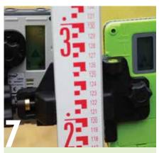
Both receivers also have a display on the rear of the unit, so the operator can stand behind the staff with the front face of the receiver facing the laser unit (otherwise they will block the beam with their body). Note the level bubble on the sliding bracket, which is used to keep the staff perfectly vertical. Also, the reverse side of the staff has 5mm increments, which is more suited to the standard receiver.
