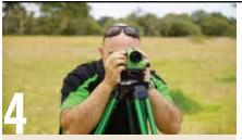
It is important not to rush this setup phase, as the accuracy of the job depends on how well the dumpy has been levelled. With that accomplished, everything viewed through the scope in line with the cross hairs will be on the same level plane.
