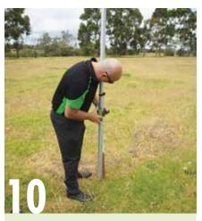
Holding the staff vertical and standing to the side or behind, slide the receiver up or down until it locks on to the laser beam
