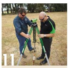
The beauty of the optical level is that it can be used to accurately set out angles or straight lines, thanks to the angle graduations on the rotary base. A common task would be to set out a line at right angles to an existing line, such as marking the locations of shed walls or squaring up a pad. Here we have placed the tripod over a corner marking peg. Note the orange plumb bob which is used to centre the tripod exactly over the peg. The dumpy is then levelled as described previously
