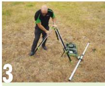
The rotary laser uses a tripod with a flat top, and is set up in much the same manner as for the optical level. Make sure the legs are well secured, and the unit is positioned away from traffic. As opposed to the optical level, the laser unit can be positioned at a lower level, as long as it is higher than all points being surveyed.
