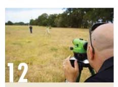
Now the unit is dialled in to the other peg which has been previously placed at the far end of our existing line. The staff is required so that the peg location can be seen through the scope.
