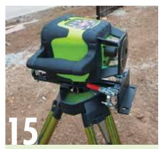
More advanced rotary laser levels have some pretty handy features. This Imex 88G can be placed on its side to create a vertical line, making it ideal for fencing. It can also do dual gradients (slopes in two directions). Gradients are not impossible with a standard unit, but just require a bit of maths
