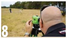
The level operator rotates the scope until the staff can be seen in the crosshairs. The small knob on the side of the base allows fine tuning of the
