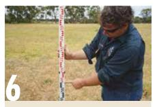
This telescopic staff is specifically designed for use with optical levels, and is known as an "E staff". Note the graduations alternate from red to black for each successive metre. The E-style graduations are designed to make it easier to view through the scope, and are grouped in 100mm blocks.
