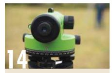
To set a line at 90 degrees to our datum line, rotate the head of the unit right (90 degrees) or left (270 degrees, as above). Any point in line with the crosshairs will now form a line at right angles to our datum.
