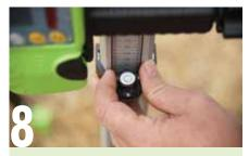
Alternatively, the staff may be fitted with its own level bubble as shown above.
