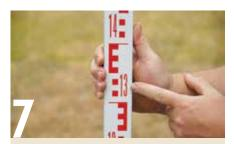
The "13" pictured indicates 1300mm from the ground or base of the staff. Each small block represents 10mm. Measurements to the millimetre are possible, but require the scope operator to interpolate between points. This means accuracy is generally plus or minus a couple of millimetres, which is adequate for most uses around the farm.
