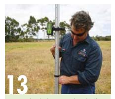
Now test the other locations. As these should all be lower than the starting point, it should be simply be a case of sliding the bottom section of the staff out until the receiver picks up the line. Subtract this reading from the original reading and you have the difference in height. For example, we recorded 1158mm at this point, so 1480 - 1158 = 322mm.
