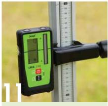
The elevation reading can then be taken, which is 920mm in this case. As long as the receiver is not bumped, the staff can be picked up and read. There is no need to hold it in position once the receiver has placed correctly.
