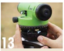
Without altering the position of the level, adjust the bezel ring so the marker is at the zero degree
