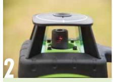
Rotating at 600rpm, the laser diode effectively creates a level horizontal laser plane. This unit uses a red diode, but green units are also available (although generally more expensive). The wavelength of the green beam is easier for the human eye to see, so it appears brighter over a longer distance. This probably only matters if you intend to use the unit inside large areas.
