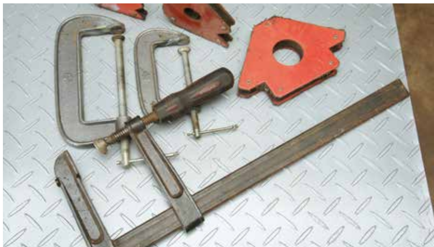
A range of G- and F-clamps will help you clamp your work during welding. Magnetic squares can also be pretty handy.
