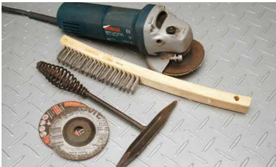
You don't need a huge range of accessories to complement your welder. A grinder with a range of grinding or flap discs is invaluable for cleaning metal and preparing joints for welding. A sturdy wire brush is handy for giving your work a quick scrub, and a quality chipping hammer is a must for removing slag post welding, and between runs.
