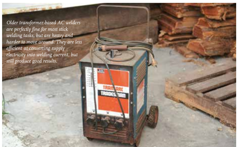
The first guide to the performance of a welder is the current adjustment knob, which displays the maximum welding current available. But be aware that the duty cycle is far more important, as it will govern how well the unit can sustain high welding currents.
