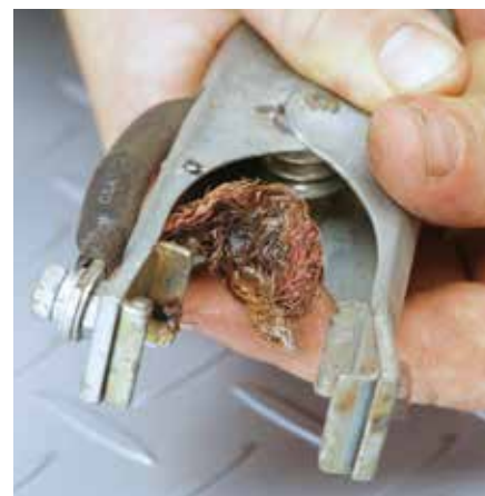
Frayed connections on welding cables increase the resistance to current flow, reducing the available welding current.
