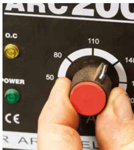
The first guide to the performance of a welder is the current adjustment knob, which displays the maximum welding current available. But be aware that the duty cycle is far more important, as it will govern how well the unit can sustain high welding currents.
