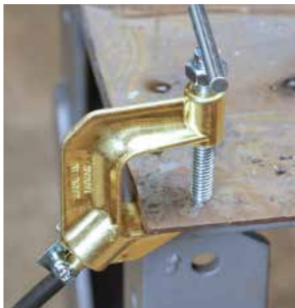
Consider upgrading earth clamps to heavy duty units, especially if your welder has a lightweight clamp fitted. This screw-down clamp is ideal for the job, but there are also magnetic clamps which make quick work of attachment.
