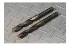
Many hand-drills have a 13mm capacity chuck, limiting the size of hole that can be drilled. One way around this is to use a reduced-shank drill bit, which has a smaller shank, usually 10mm or 12.5mm, allowing it to fit into a regular chuck. But problems may arise with slippage when using large diameter bits. Drilling speed will also need to be reduced as diameter increases.
