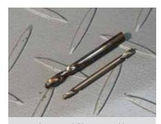
Rivet or thin section drill bits are suited for drilling shallow holes in thin materials such as sheet metal and are available in bright, blue and titanium nitride coated high-speed steel and cobalt-steel alloy. The 135 degrees point angle minimises breakthrough damage on the drill lip edge, and reduces wandering. Sizes to suit 3mm, 4mm, 1/8, 5/32 and 3/16 inch rivets are commonly available in double-ended, single-ended and stub drill configurations.
