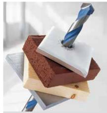
There are a few different styles of multi-purpose drill bits featuring a tungsten carbide tip. These Bosch multi drills are a good example, and can handle concrete, masonry, wood, sheet metal, aluminium and ceramics, and can be operated with or without impact. They are handy when you need something to handle a range of jobs, but don't expect the drill to bore an accurate size hole.
