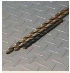
While HSS drills are available in long series for deeper holes, ultra-long drill bits are available for applications where extreme drilling depth is needed. These drills are not easy to use and must be handled very carefully. Drills have a tendency to wander and not drill straight and must be withdrawn to clear swarf often because clogging is a real issue. Use low feed pressure and lower drilling speeds. They are also ideal where drilling access is limited.
