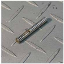
Dedicated glass drill bits have a fine layer of diamond grit attached to the cutting edge and the sides of the bit. The layer of grit is attached using either electrolysis for cheaper drills, or sintered on using high temperatures for the better quality bits. They require a flood of water during drilling for cooling and lubrication. For drilling on vertical surfaces, you can use a small stick-on plastic tank to hold the water, which is often supplied with the drill bit.
