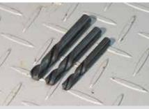
Left-handed drill bits are specifically designed for drilling out broken bolts and studs, and are used with drills set in reverse rotation. The contrarotation of the drill bit often helps to loosen the stub of broken bolts. They are available in standard lengths, or short lengths as pictured, which have less tendency to snap. The blue colour, which is common to some HSS drill sets, is a ferric-oxide coating, which helps reduce chip welding and heat build-up, in a similar fashion to TiN coatings.
