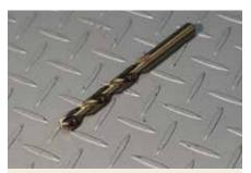
Cobalt drill bits have five percent cobalt added to the HSS alloy, resulting in extended cutting life between sharpening. They look similar to standard HSS drill bits, but are often marked with 'HSS Co' on the shank, and the split point is ground to 138 degrees. They are primarily used for drilling tougher materials including stainless and high-tensile steels, and cast materials which may have a hard surface skin. They can cost up to three times the cost of standard HSS drill bits.
