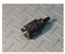
If you need to drill larger diameter holes in ceramics, for example to fit a tap through the bathroom wall, a good option is a diamondtipped core drill, which is basically a holesaw for ceramics. There are several styles of these core drills with coarse or fine embedded diamond grit, and depending on the manufacturer, some versions can drill glass.
