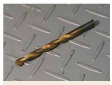
The gold-coloured coating seen on many drill bits is titanium nitride (TiN), which increases the surface hardness, improves abrasion resistance and helps prevent the tendency for metal chips to cold-weld themselves to the surface of the bit. The TiN coating is supposed to reduce friction, allowing the bit to be used at speeds of up to 20 per cent over that of a standard HSS drill bit, or alternately an increased feed rate.
