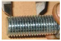
For Imperial threads the thread size is expressed as the number of threads per inch. Here we have used the thread gauge to measure 13 threads per inch on this ½ inch bolt.
