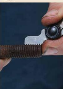
Metric threads are specified by the distance between adjacent threads, which is called pitch (see Figure 1). From the thread tables (pages 139 to 141) we know that an M16
