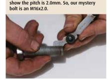
A tap and die set can be used as a set of thread gauges to match the pitch or TPI of metric or imperial threads.
