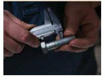
Match the bolt threads to the thread tap as shown. If the tap is in good condition you should be able to read the pitch straight off the shank of the tap.
