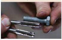
Whitworth threads can really upset the apple cart. They often have the same TPI as UNC threads (see thread tables), but use a different thread angle of 55 degrees, whereas UNC and UNF use 60 degrees. While many will be found to be interchangeable they may feel loose or tight in the threads due to the difference in angles. One size that will invariably trip you up is  $\frac{1}{2}$  inch UNC and BSW. They look very similar, but the  $\frac{1}{2}$ " BSW has 12TPI (right).
