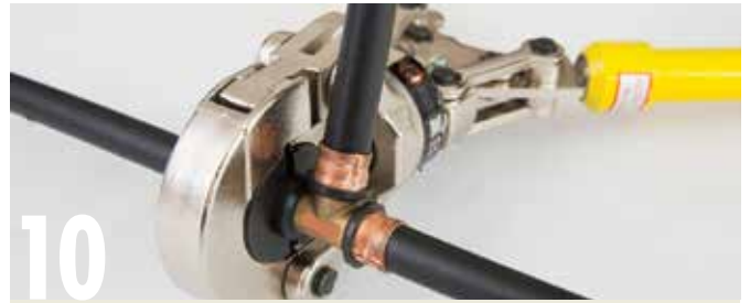
While Sharkbite fittings are the most convenient, there are several types of fittings used to join PEX pipe, including crimp and compression-style fittings. Auspex iCrimp fittings have a small copper sleeve around the outside of the pipe. The pipe is pushed into the sleeve until it can be seen through the small sight hole on the inner edge of the sleeve. The sleeve is then crimped on using the proprietary crimping tool.
