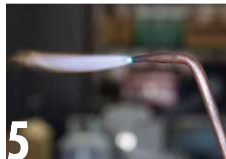
5 A heat supply is the next thing needed, and most farmers will turn to the oxy-acetylene set, which is more than capable of providing enough heat for the job. Use a smallish tip and adjust the flame to neutral. Oxy-LPG or MAPP gas will also work, but LPG or propane by itself will not be hot enough.
