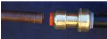
Incredibly, there are also Sharkbite fittings for joining copper pipe, which work in much the same way as the PEX pipe fittings. The most notable difference, other than the orange colour plastic sleeve, is the absence of the internal sleeve as used with the PEX fittings. The 1/2" copper joiner costs about $4.40 and the 3/4" joiner costs about $7.15.
