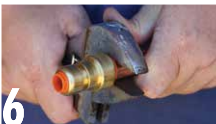
A shifter spanner makes a great improvised removal tool for both PEX and copper Sharkbite fittings.
