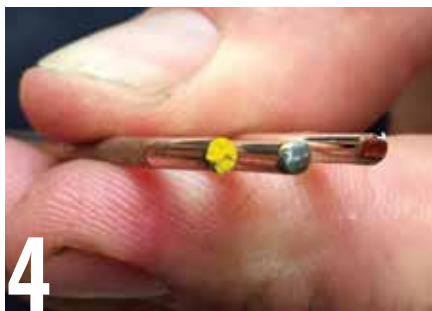
4 Silver solder is actually a brazing alloy, and is available in a range of different alloys, or compositions of metals. For standard silver soldering of copper fittings, a 2.5mm yellow-tip, 2% silver rod is adequate (about $3). The grey tip is 5% silver and the brown tip is 15% (and about $15 a rod).
