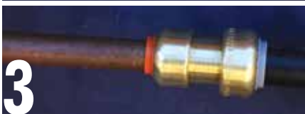
As with the PEX pipe, installation is about as simple as it gets. Simply push the tube into the fitting, making sure it goes in full depth past the restriction of the O-ring. Note the fitting above is a combination joiner for attaching PEX pipe (grey sleeve) to copper pipe (orange sleeve). It costs about $4.40.
