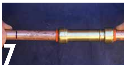
This slip coupling is great for repairing a leak in copper tubing, or joining two tubes where the ends are not quite close enough. If a pipe has developed a split, the damaged section can be cut out with a tube cutter. The slip end (opposite to the end with the ring) can be pushed down over a tube, then pulled backwards onto the other end with the use of a removal tool.
