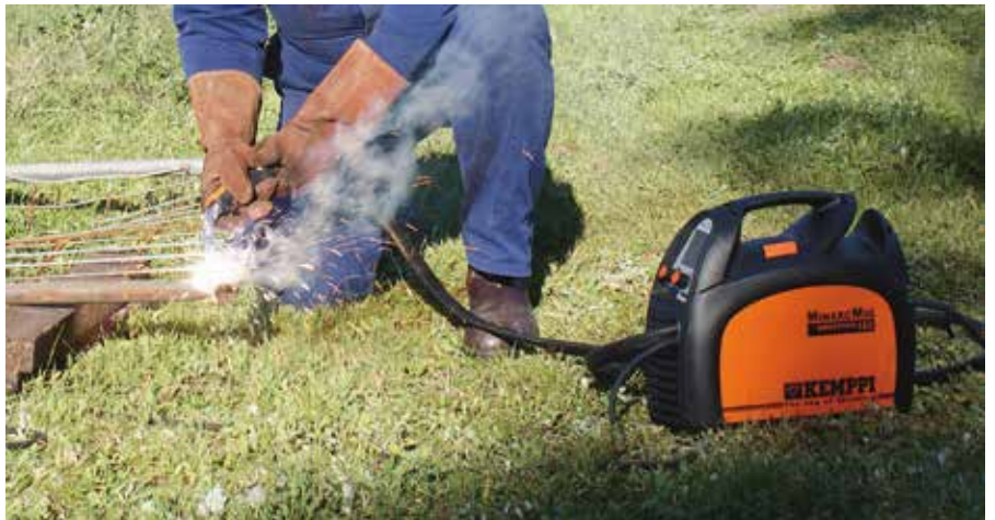
While many MIG welders use shielding gas and are confined to indoors use away from the breeze, a new range of ultra-portable units have hit the market. These are ideal where extreme portability is required, and can be used outdoors with flux core wire, which produces its own shielding gas.
