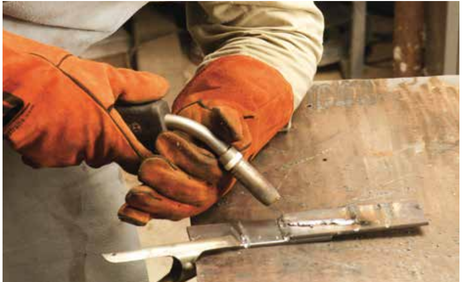
MIG welders allow the operator to use both hands on the welding handpiece for greater control.
