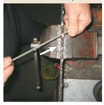
If the chainsaw is cutting skewed, the teeth are likely to be longer on one side of the bar than the other. This needs to be rectified quickly, as the links and the bar will wear unevenly, causing skewed cutting despite a correctly sharpened chain. Use a vernier calliper (pictured) to compare teeth lengths. A crescent spanner also can be used. To align tooth lengths, give the longer teeth a few more strokes with the file than the shorter teeth.
