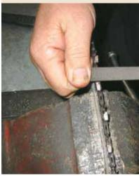
After lowering the depth gauges to the required height, round the leading edge of the raker with the file as pictured.
