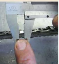
As the chainsaw teeth are filed back, their height decreases, which will reduce their cutting performance. Every so often it will be necessary to lower the rakers or depth gauges. These are the rounded forms in front of the teeth that control the depth of tooth engagement in the wood. Pictured are a flat depth-gauge file and a height gauge.
