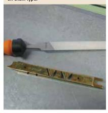
1 O File the gauges in the same direction as the teeth are sharpened. Only a few strokes will be needed to file the depth gauges to the required height.
