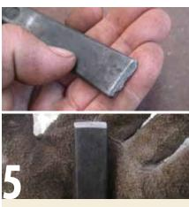
With the wheel dressed, a few spare minutes can be put to good use sharpening blunt cold chisels or drill bits, but remember to cool often in a cup of water.
