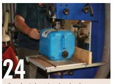
Clean chemical containers have long been a handy source of storage for the farm workshop. Just make sure they really are clean and have not held anything toxic. A bandsaw (above), jigsaw (below) or even an angle grinder with thin disc can be used to cut them with relative ease.
