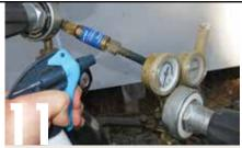
Fill another spray bottle with a mixture of water and dishwashing liquid. Spray it around oxyacetylene fittings and hoses to check for leaks. They may be small, but a slow leak will cost dollars over time.
