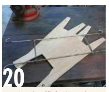
Extension cords are difficult to tidy up at the best of times. Here are two different types of cord-tidies you can make in minutes; one from galvanised rod and one from ply board.
