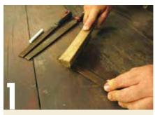
Poor old hand files never seem to get any attention. They work so much better if they are regularly cleaned, by scrubbing along the serrations with a wire brush or file cleaning card.
