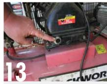
It also pays to check compressor oil levels and drain any moisture from reservoirs and water traps. These jobs are typically overlooked until a problem crops up.
