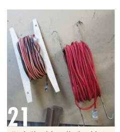
Note the tidy made from rod has the ends bent over so it can be hung up, while the one cut from ply has a hole drilled for hanging.
