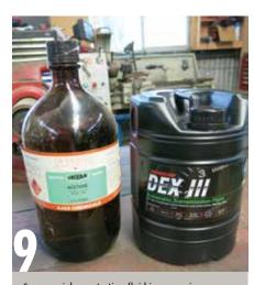
Commercial penetrating fluid is expensive (\$50 for 4 litres) but a very good, possibly superior substitute can be made by mixing 50:50 mineral automatic transmission fluid (unused) and acetone. While diesel or kerosene makes a reasonable substitute for a commercial penetrating fluid, the ATF/acetone mix has a superior ability to wick into seized parts.
