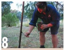
Give handles a liberal coating with an old paint brush. The turps helps thin down the boiled linseed oil, helping it soak into the handle. Don't use raw linseed oil as it will take ages to dry, and may remain sticky. The boiled linseed/turps mixture should be dry in about a day.
