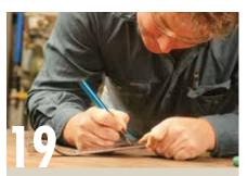
Marking tools for security is another good job to chip away at when you have a few spare minutes. This Kincrome pen engraver has a hardened tip, ideal for marking spanners, and costs around \$39.
