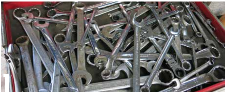
1 This drawer full of metric spanners includes ring, open-end, combination ring/open-end and ratchet spanners. It is hard to find anything in a hurry, with many spanners looking the same, and larger spanners obscuring the smaller spanners.
