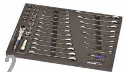
2 The standard in tool trays these days is EVA foam inserts, offered by manufacturers such as Kincrome. This is all well and good if purchasing tools from new where the trays are included, but basically impossible to purchase a tray for pre-existing tools. Note that even though this tray is well laid out, it is not particularly space efficient.
