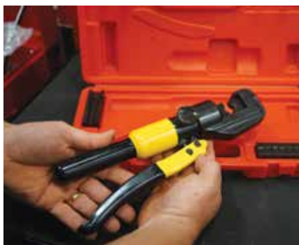
Back in June's workshop we looked at installing battery terminals using a hydraulic crimping tool. This Matson unit handles lug ends from four to 70mm 2 and costs $100.
